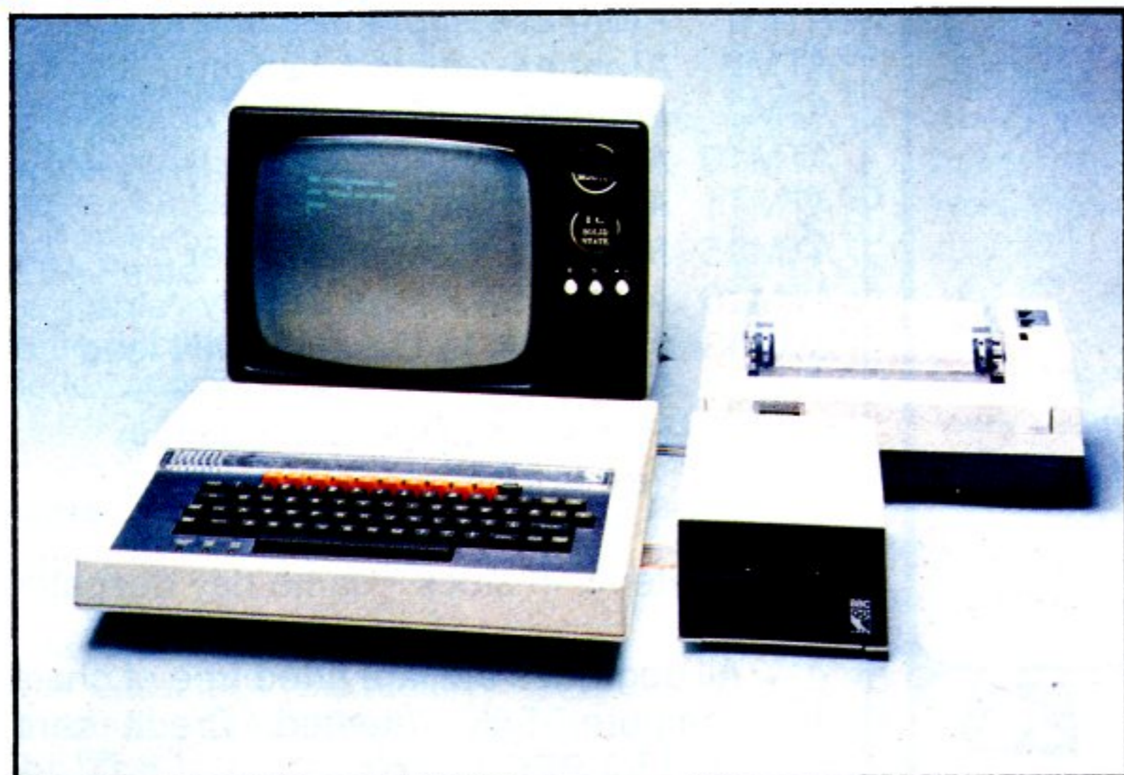
BBC micro with single disc drive and printer. The cover shows a BBC micro with a double disc drive.
