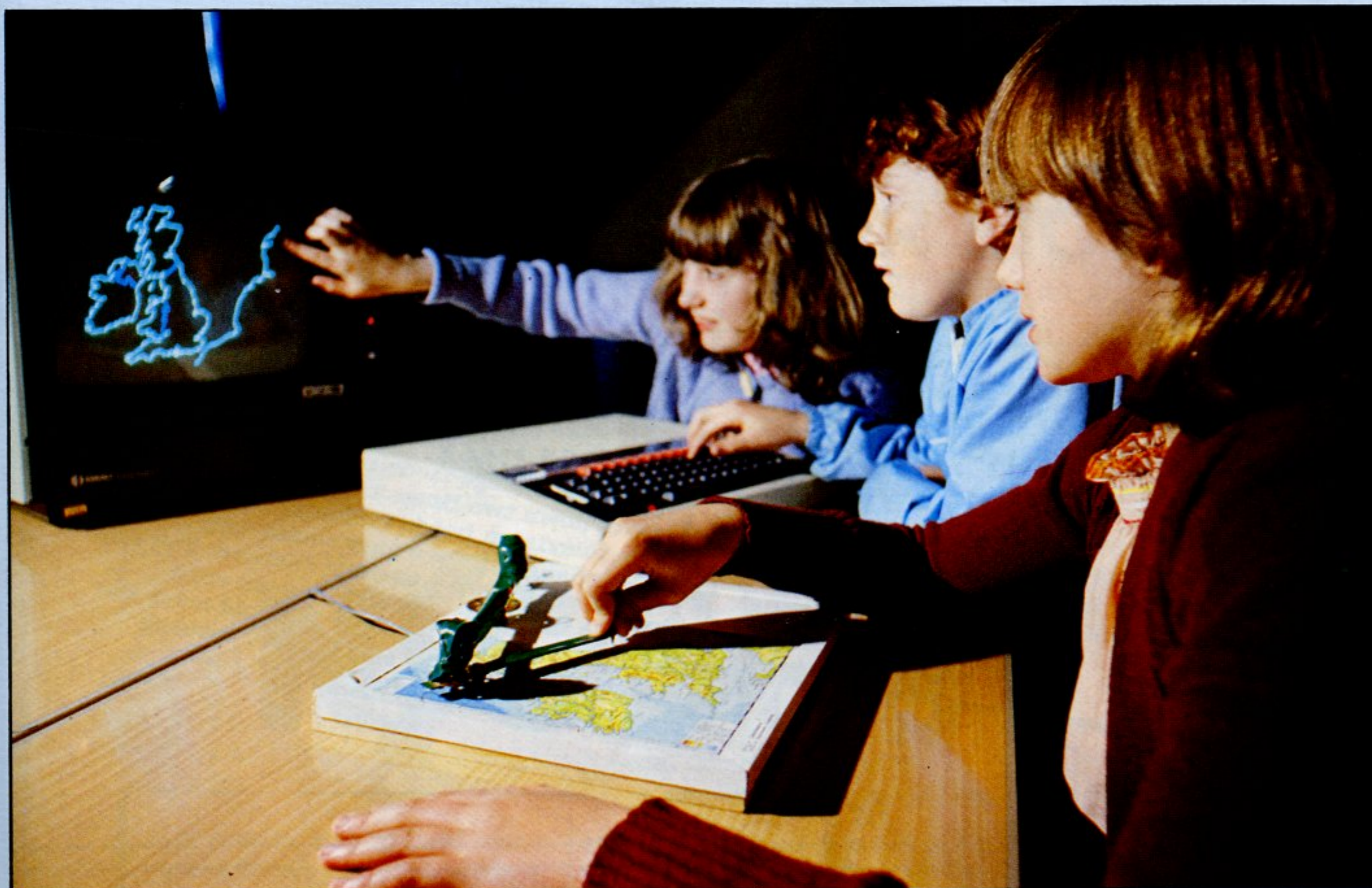
The pupils are using the Cambridge Local Education Authority device which enables them to trace a picture from a book or map directly onto the screen of the BBC micro.
